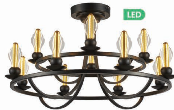
Model No. : MZD940-D0.2×1368-WYT-YASI Dimension : Ø940 x 540mm Power : 90W (LED) Color Temperature : 2700K-5700K
