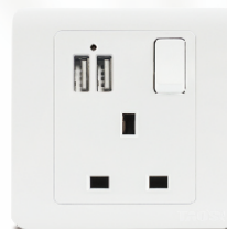
71456 13A 1 gang switched socket, DP + 2*USB (2.1A shared) +neon (switch controls USB)
